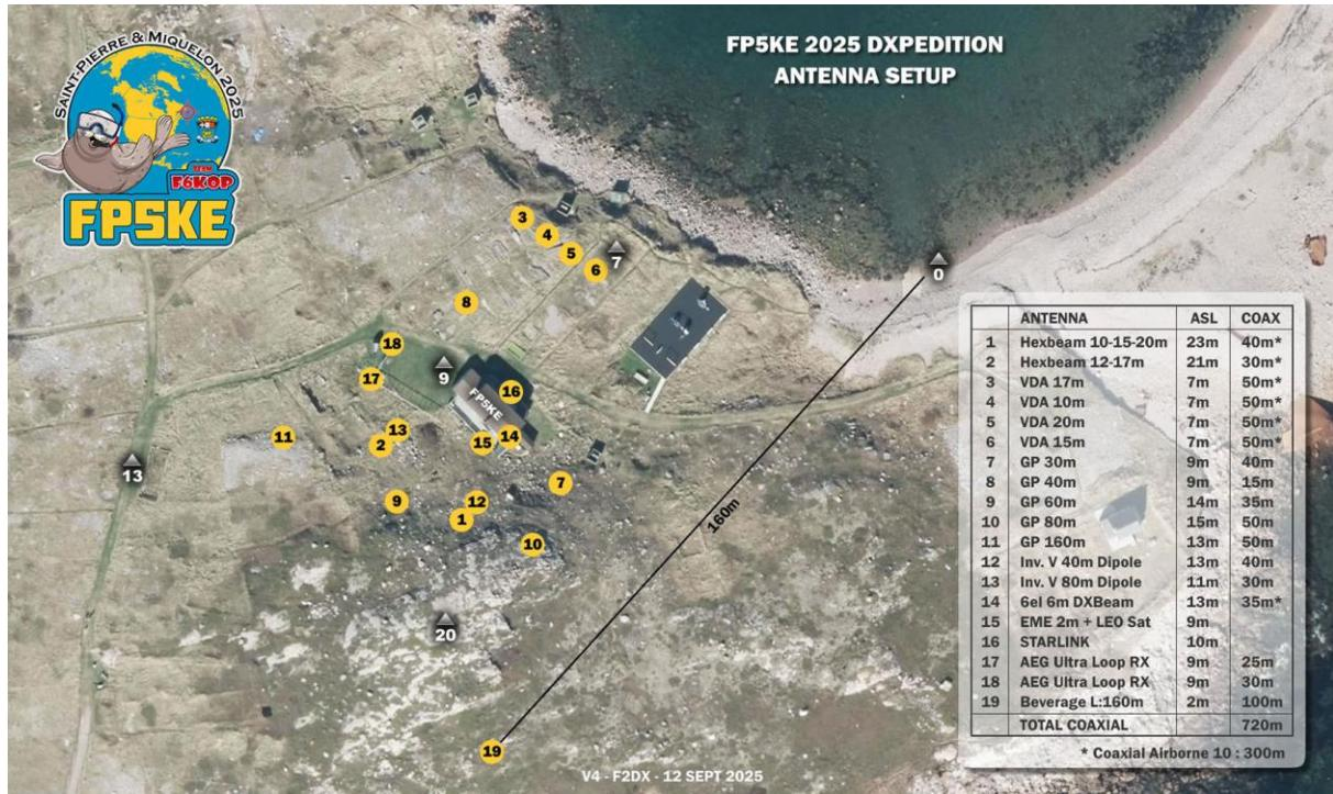
This setup gives us two antennas on each HF band, enabling true *in-band* operation (two stations working simultaneously on the same band in different modes). This is made possible by adequate antenna spacing, opposite polarization, and band-pass filters. For low-band reception we added three highly effective antennas: two Vertical-Array loops and a 160-meter Beverage, using a kit supplied by SO9I Engineering.
