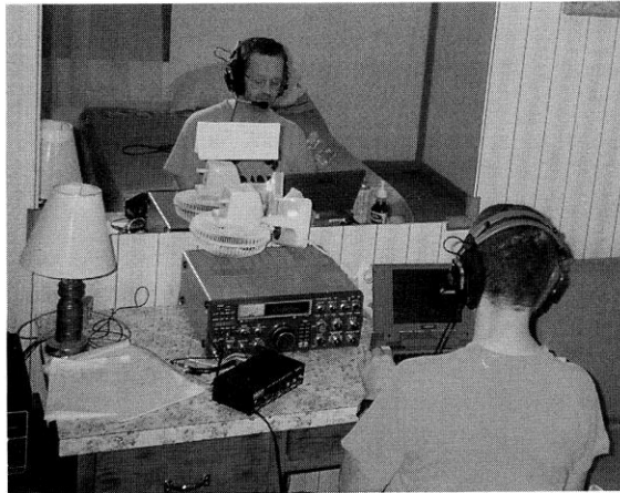
Dave, W5AO, (T88M) finally on the air. Note the "external" cooling fan on the TS-930.
